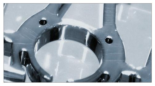
Precision electroforming is an additive process in which 2-D and 3-D microstructures are formed by electrochemically depositing metal into a precisely formed photoresist mold. Electroforming is ideal for fabricating micron-scale, metallic components as well as for making injection molds used for forming nonmetallic microstructures with nano-scale features.
